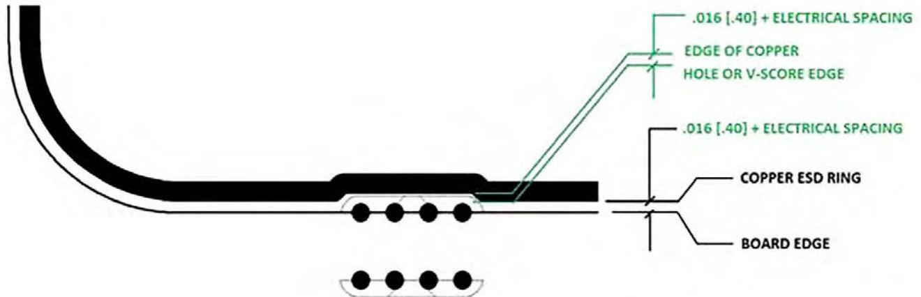
Figure 6: Recommendations for minimum copper-to-edge clearance.
