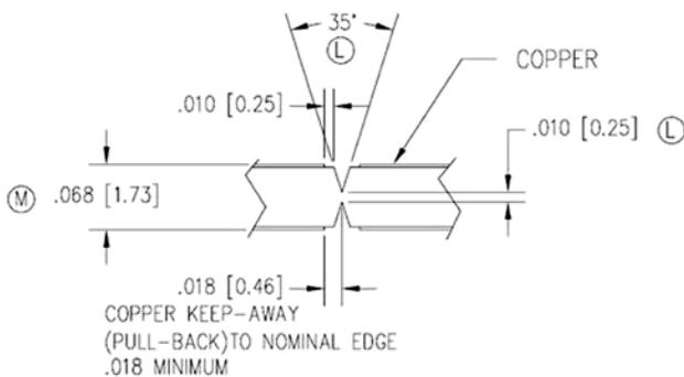
Figure 9: V-score scenario showing copper pull-back requirement at worst-case least/max material conditions.
