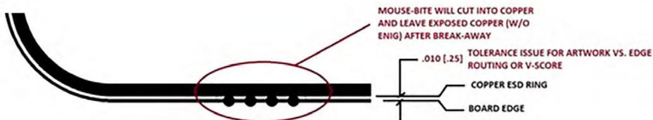
Figure 1: Example of insufficient copper-to-edge clearance.
