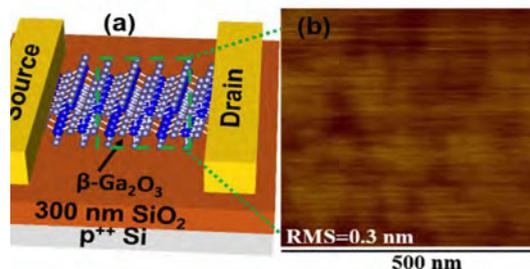
from beta gallium oxide have a higher "breakdown voltage," or the voltage at which the device fails, said Professor Peide Ye of Purdue University.
