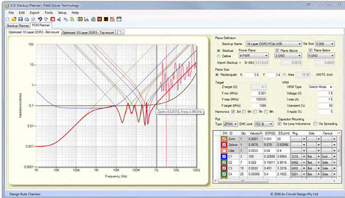
Figure 4: PDN analysis of the bottom mount decoupling capacitors.
