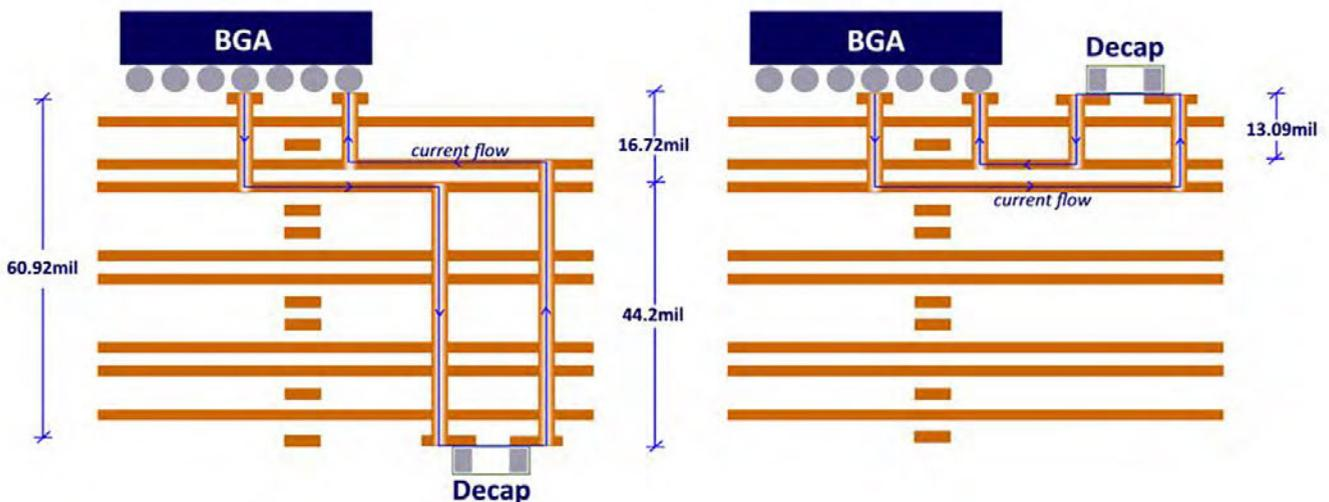
Figure 3: Decoupling capacitors placed on bottom vs. top of board.
