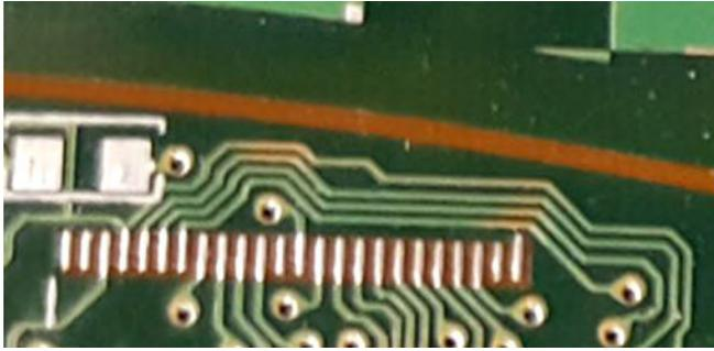
Figure 7: A nearly complete PCB, prior to routing.
