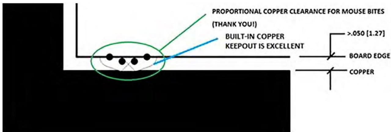
Figure 3: Example of robust copper-to-edge clearance on a low-density design.
