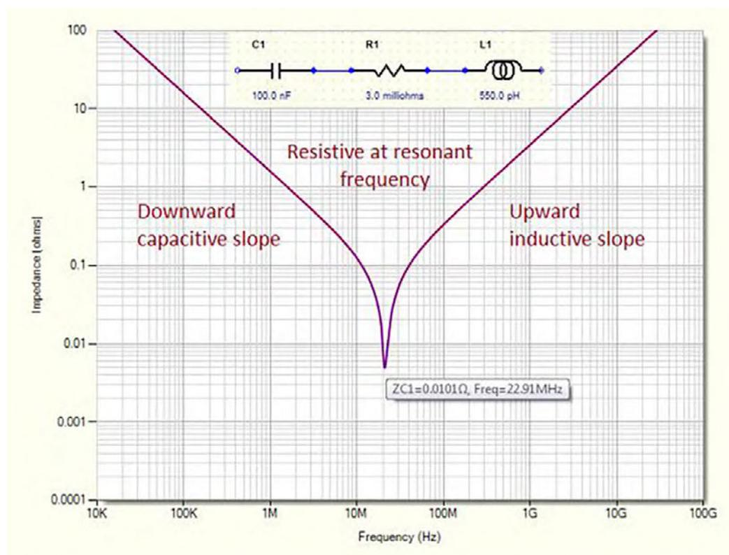
Figure 1: A capacitor has series capacitance, resistance and inductance.
