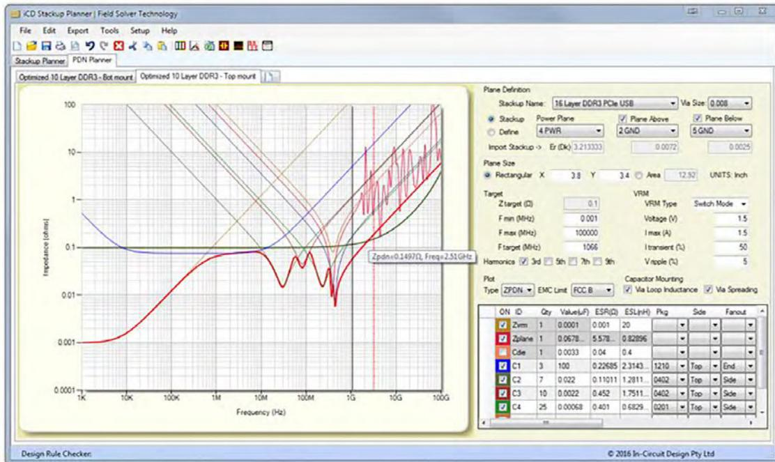
Figure 5: PDN analysis of the top mount decoupling capacitors.
