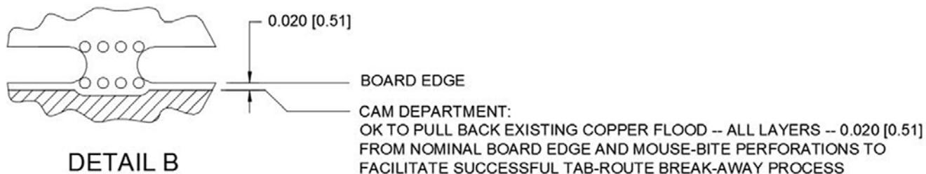
Figure 2: Fab note allowing CAM department to modify copper-to-edge spacing.
