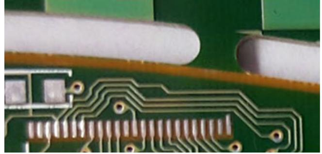
Figure 8: Example of board with tab only due to close proximity of traces.
