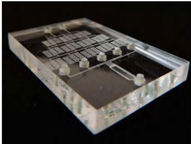
"Microfluidic chips are advancing point-of-care diagnosis for many diseases," says Alicia Toh from A\*STAR's Singapore Institute of Manufacturing Technology (SIMTech). "Inside these chips, tiny microvalves precisely direct microlitres of fluid through a series of microchannels for automated analysis. However, integrating microvalves into the microchannels is complex and highly susceptible to fabrication defects, which translates into a higher cost per device."
